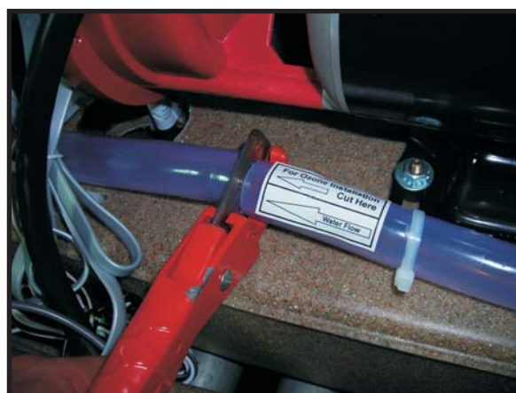
2. Cut Hose next to the ozone installation label
